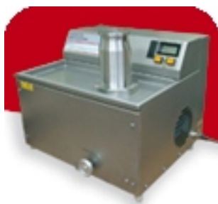
Fig. 2. High-pressure homogenizer (One Shot Model, Constant Systems Ltd.).
