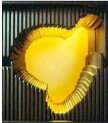
Fig. 3. Multi-leaf collimator – the position of individual leaves defines the shape of the irradiation field.
