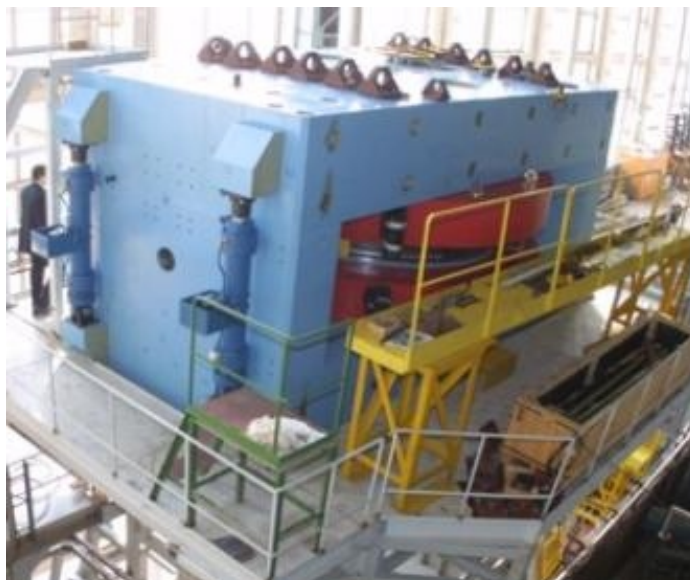
Fig. 12. Cyclotron DC-72 with a maximal energy of protons of 72 MeV constructed in Dubna for the Cyclotron Centre of the Slovak Republic. One of the intended applications of the cyclotron is proton therapy of eye tumours.
