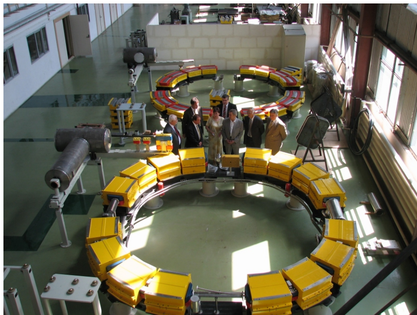
Fig. 13. Medical proton synchrotron for Slovakia at the construction site in Protvino, Russia.
