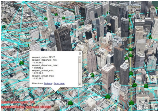
Fig. 5. Simulation run of on-demand transport coordination scenario exported in KML format and displayed by Google Earth. The input benchmark was based on historical traffic and demand data from San Francisco, 2008.
