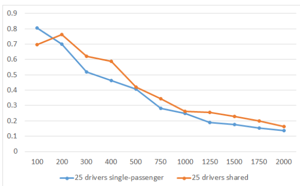
Fig. 8. Success rate comparison of single-passenger and shared taxi service with 25 vehicles. Horizontal axis corresponds to number of requests per day, while vertical depicts the success rate (success rate of 1 would mean that all the requests are served).
