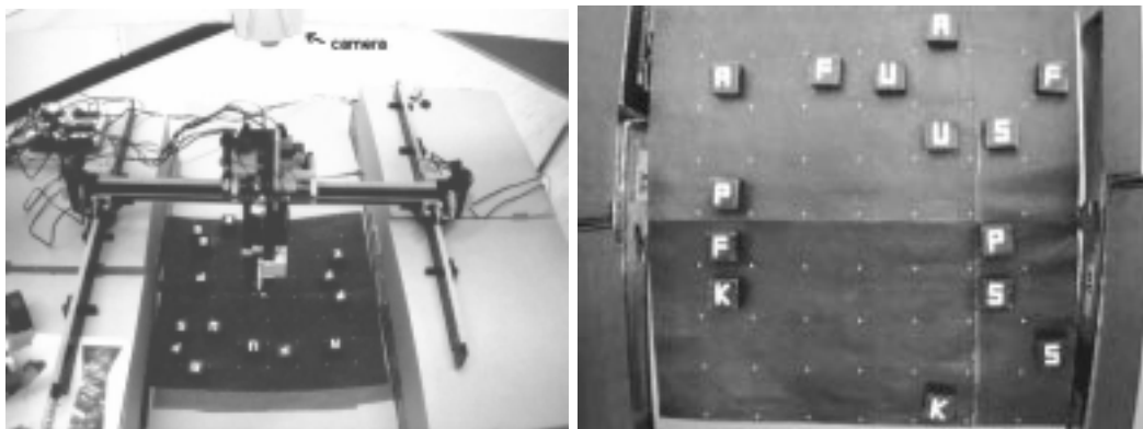
Figure 3. Gantry robot (left), view from the camera (right).
