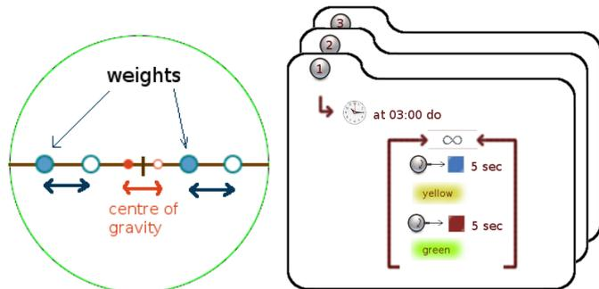
Figure 1. Principle of autonomous ball movement (left), concept of the programming paradigm: Iconic language, multiple balls, events, control structures (right).
