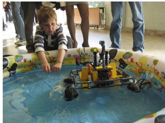
Figure.1. Boat robot for Istrobot contest. Capable of navigating 100s of meters across a lake using compass sensor.
