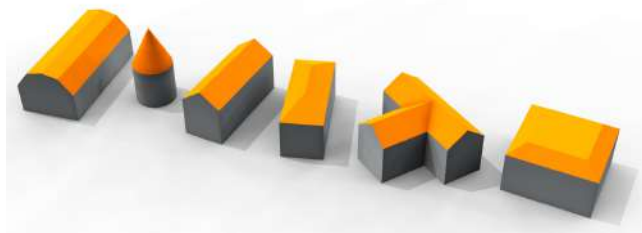
Figure 7: Selected roof types. From left to right: gambrel, cone, gabled, hipped, cross-gable, mansard.
