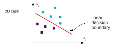
Fixed-increment convergence theorem (Rosenblatt, 1962): "Let the classes A and B are finite and linearly separable, then perceptron learning algorithm converges (updates its weight vector) in a finite number of steps."
