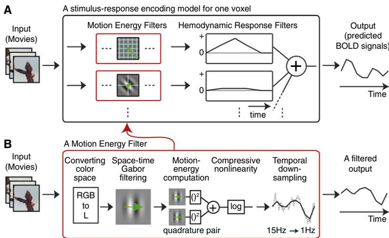
Figure 1. Schematic Diagram of the Motion-Energy Encoding Model
